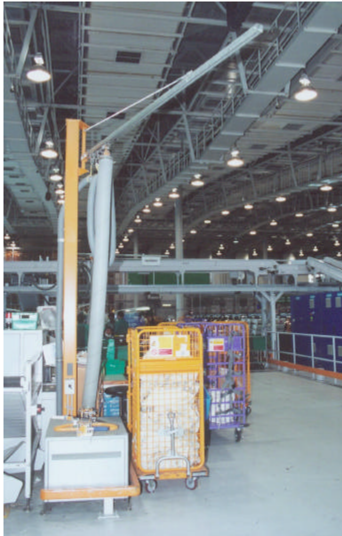
Photograph 6 Vacuum lifting device
